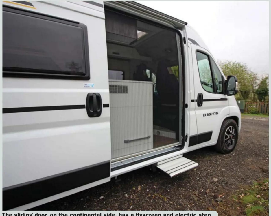
The sliding door, on the continental side, has a flyscreen and electric step
