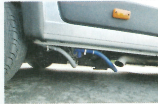
Water-tank drainpipes dangle and are close to the exhaust
