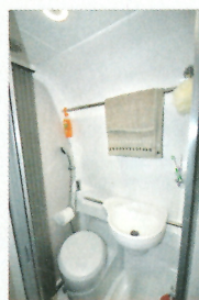
Tambour door saves space; handbasin slides over for more room when showering
