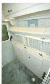
Seat/bed frames fold away to optimise storage space just inside the back doors
