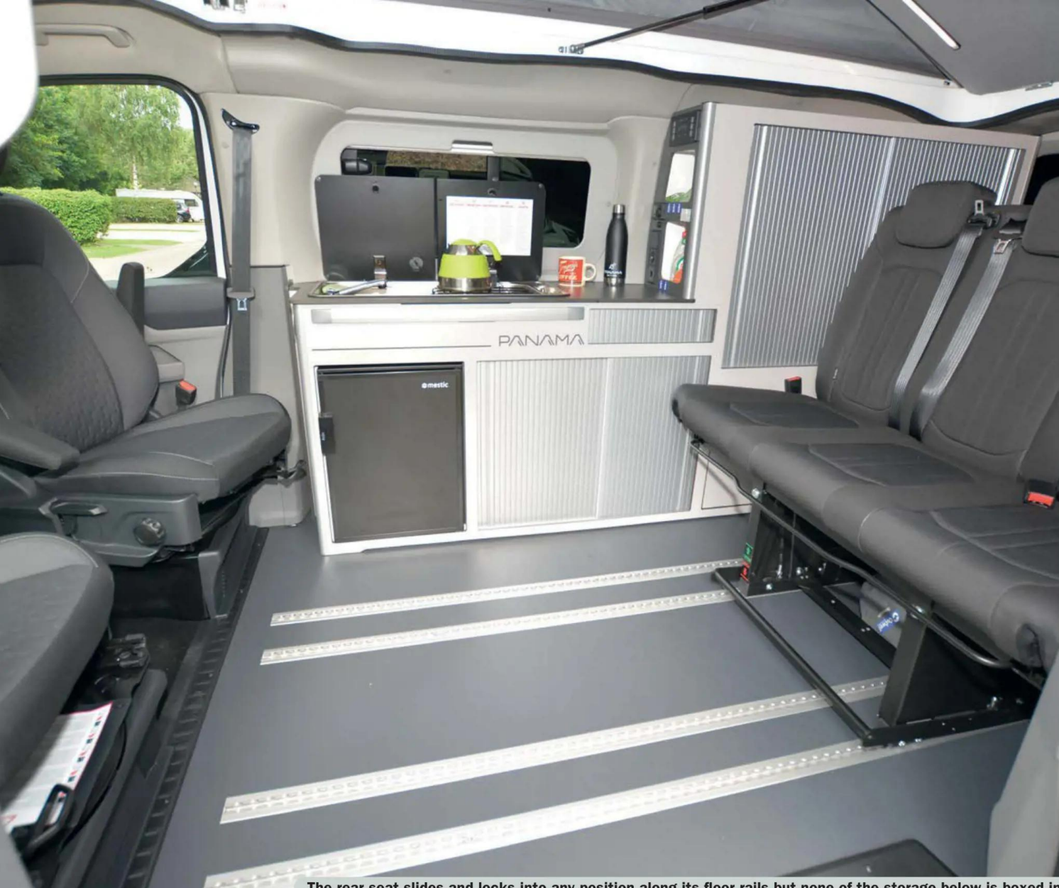
The rear seat slides and locks into any position along its floor rails but none of the storage below is boxed in
