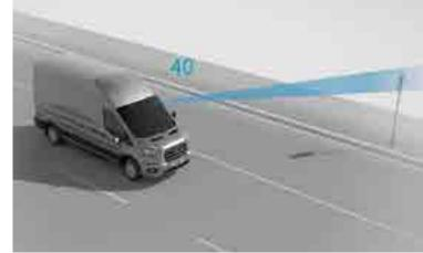
**TRAFFIC SIGN RECOGNITION** Whether the signs are at the side of the road or above it, permanent or temporary, Traffic Sign RecognitionØ1) can identify them. An icon of that speed or no-overtaking sign appears on the instrument cluster and changes every time you enter a new limit, keeping you fully informed on every
