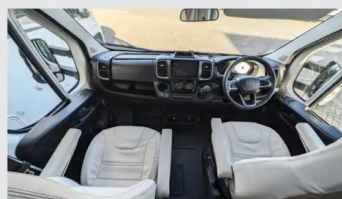
Standard Fiat Ducato cab, with captain's chairs that swivel to form the lounge
