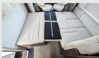
Generous double is made up by lowering the table and folding down the side seat
